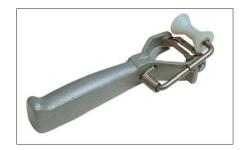
IT-1000-030-2 Screen Removal Tool Tyco Electronics Screen Removal Tool IT-1000-030-2 for bonded screens on round conductors of MV Cables, incl. 1 spare blade, silicone grease and allen key delivered in a robust polypropylene box. Suitable for one and three core cables.
